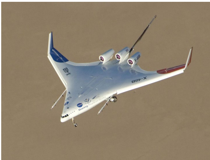
Figure 3. X-48B blended-wing body. (From NASA Dryden Flight Research Center Photo Collection, 14 August 2007, http://www.dfrc.nasa.gov/Gallery/Photo/X-48B/Medium/ED07-0192-08.jpg .)
